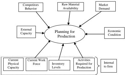
Fig. 1 Required Inputs to the Production Planning System.
